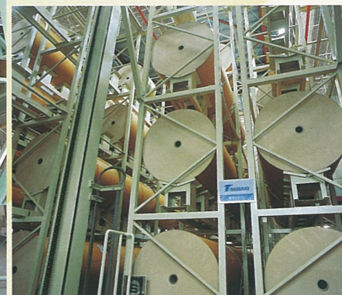
立体紙庫から直接移載 Direct transfer from vertical storage yard
