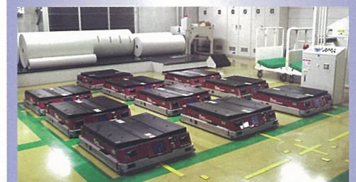
充電待機中のADS ADS waiting for battery recharge
